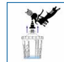
STEP 6 dismantle the cup from the spraying gun
