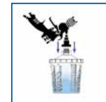
STEP 4 turn the gun 180 degrees and push it onto the sieve opening
