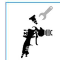
STEP 1 install the appropriate adapter on the spraying gun
